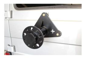
**Step 4:** Install spare tire with new wheel bolts in the following order: Start all the bolts, then hand tighten all bolts, then torque the bolts to at least 70 lb. ft.
